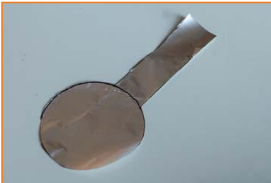
Figure 3. The all-DIY capacitive sensor.
