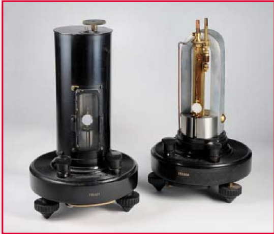
Top Hat Galvo. The Leeds & Northrup 'top hat' galvanometer is familiar to anyone who worked in yesterday's scientific laboratories. It detects tiny electrical currents by using a beam of light as a long, massless pointer. It's about 8" (20 cm) high. Today's galvos are mostly used in scanning applications. They are much smaller, more rugged, and orders of magnitude faster. Photo courtesy of Conrad R. Hoffman.
