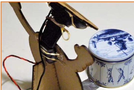
Figure 4. Detail of Cookie Guard's neck construction.
