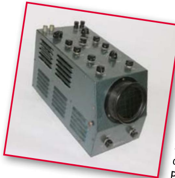
Top Hat Galvo. The Leeds & Northrup 'top hat' galvanometer is familiar to anyone who worked in yesterday's scientific laboratories. It detects tiny electrical currents by using a beam of light as a long, massless pointer. It's about 8" (20 cm) high. Today's galvos are mostly used in scanning applications. They are much smaller, more rugged, and orders of magnitude faster. Photo courtesy of Conrad R. Hoffman.
